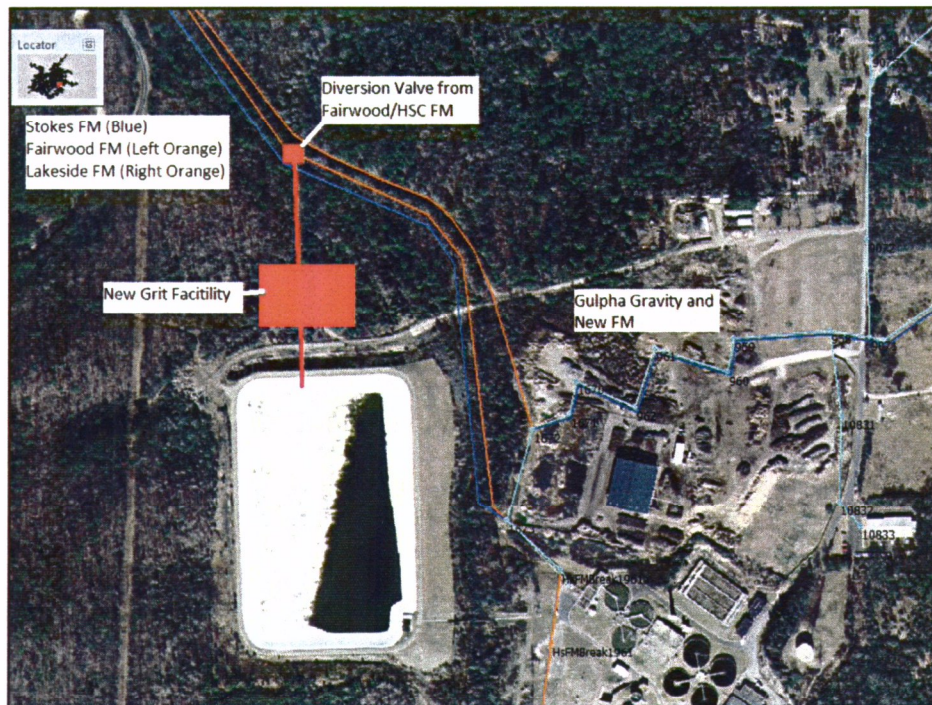
Figure 4.17: New Grit Removal System Location #1
